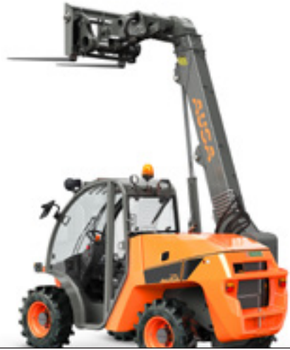
T235H 5,000 lb MAXIMUM LIFT 16.4 ft POWER 44.5 hp WIDTH 62.6 in TRANSMISSION HYDROSTATIC
